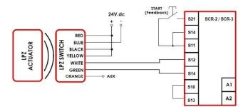
Single switch to SCR-31P-i Safety Relay (Viper series):
