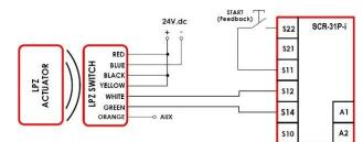
Multiple switches to SCR-31P-i Safety Relay (Viper series):
