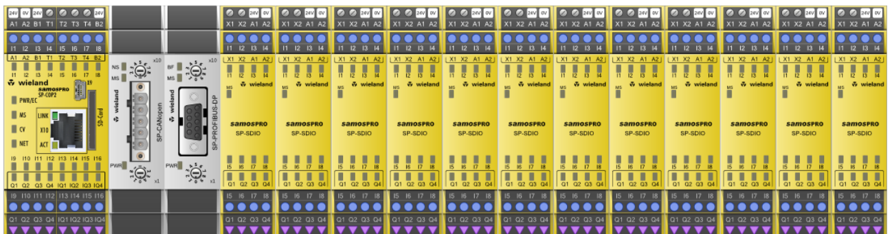
Illustration 3: Example 2 - Maximum expansion of a samos®PRO system
