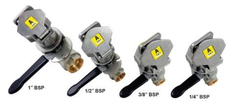
IDEM's mini valve locks can be used standalone or for use as part of a SKORPION Trapped Key solution. They can be locked in an open or closed state (passing or non-passing). The key can then be removed and can be moved to safe storage (to avoid tampering) or can be integrated with trapped key guard interlocks to protect operators from machine, gas or air hazards that may be present.
